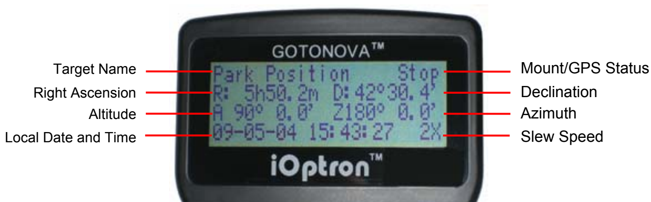
Figure 2. #8405 Hand Controller LCD Information Screen
