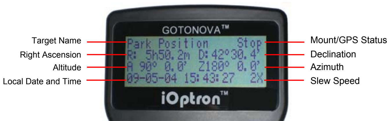
Figure 2. #8405 Hand Controller LCD Information Screen
